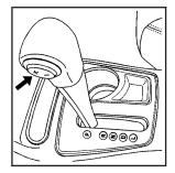
This feature allows you to limit higher gears by selecting a maximum gear range when the shift lever is in LOW (L). The button for this mode is located on the left of the shift lever knob.
